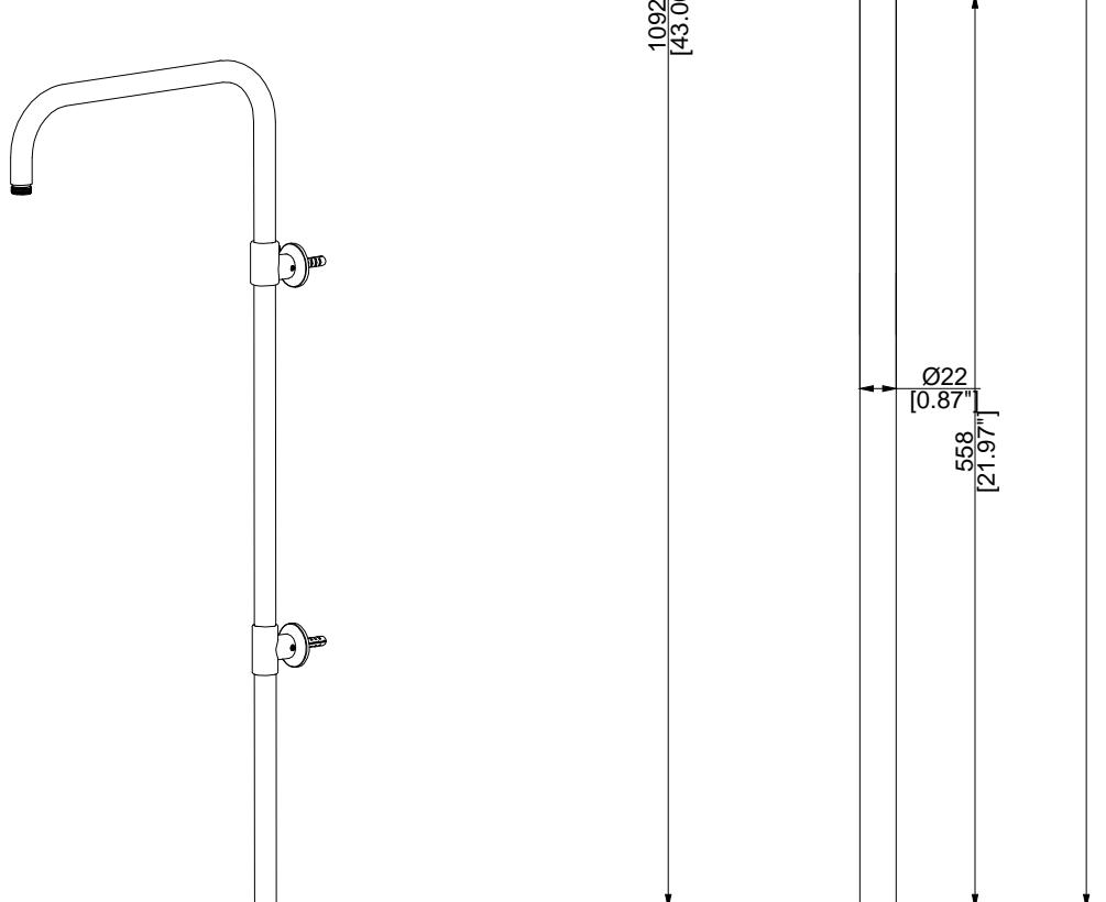
Bottom section below fixed wall bracket can be cut to obtain desired height
